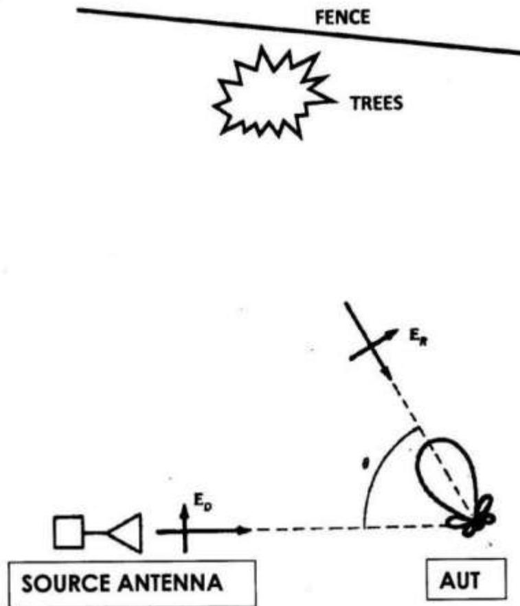
Figure 6.6 Amplitude of the spatial interference level for a given reflectivity level and antenna pattern level
