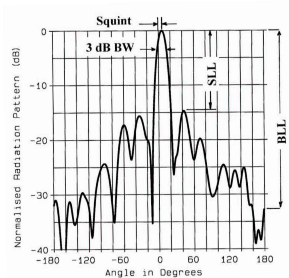
Figure 8.2 E-plane patterns of 1.22 m diameter source dish for S band with  $0^\circ$  and  $180^\circ$  receive polarization before alignment
