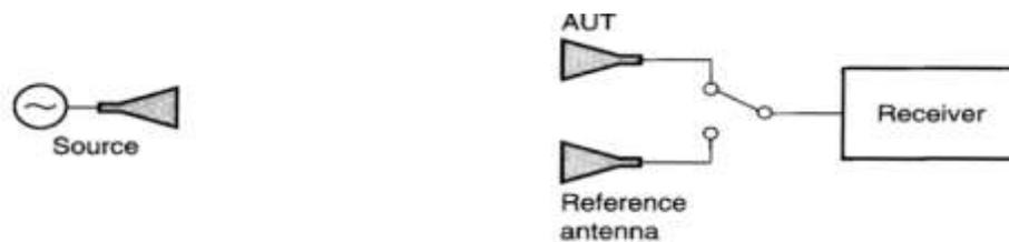
Figure 4.1(b) Test set-up showing AUT and gain reference mounted back-to-back (note absorber to eliminate reflections into gain standard)
