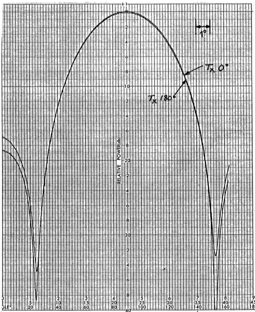
Figure 8.4 H-plane patterns of 1.22 m diameter source dish for S band with  $90^\circ$  and  $270^\circ$  receive polarization before alignment
