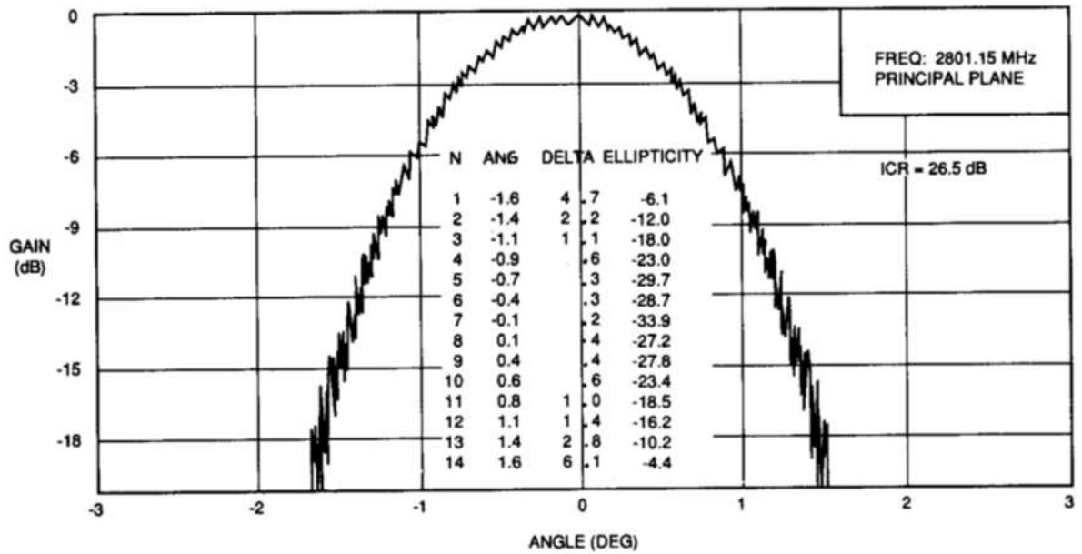
Figure 5.6 Relationships between axial ratio (ellipticity) and cancellation ratio
