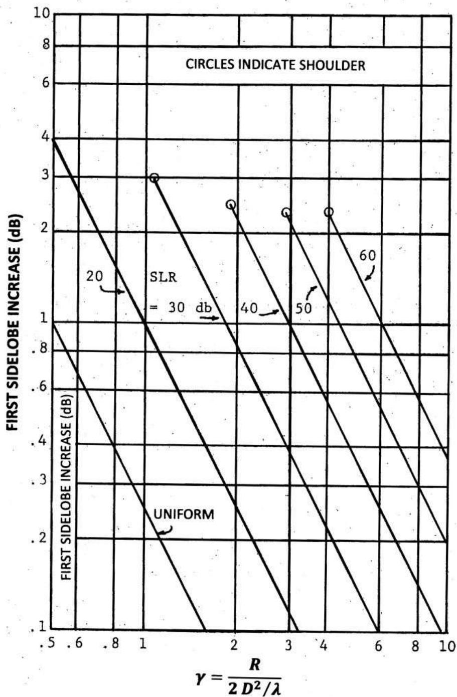
Figure 6.4 Effect of amplitude taper in the test field
