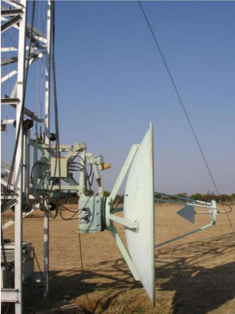
Figure 2.10 Synthesized sweeper with DC power supply on top, fibre optic control link at left and Mini Circuits amplifier at right
