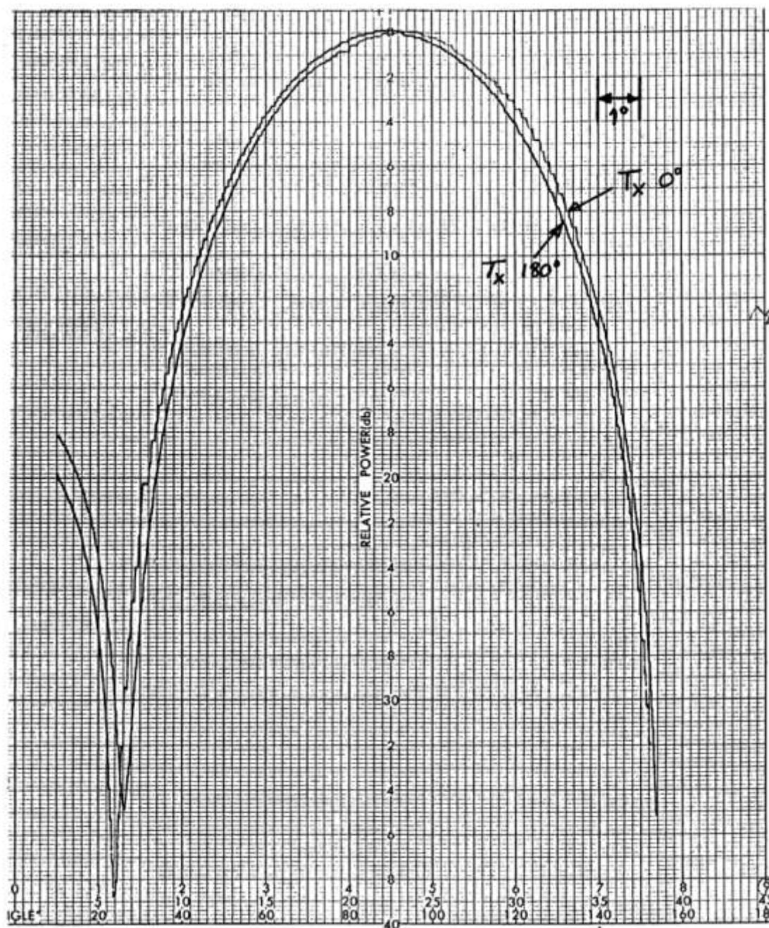
Figure 8.3 E-plane patterns of 1.22 m diameter source dish for S band with  $0^\circ$  and  $180^\circ$  receive polarization after alignment
