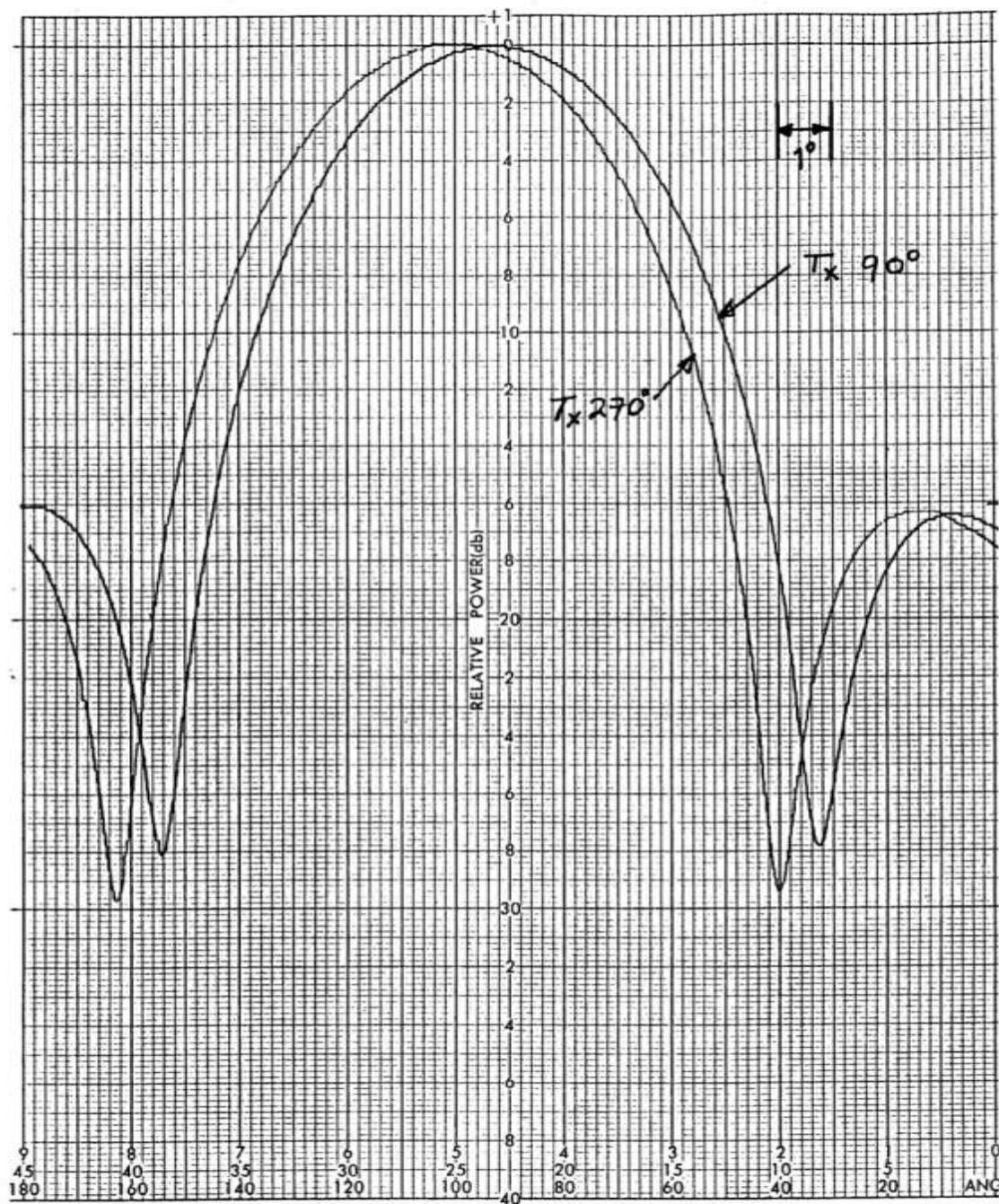
Figure 8.5 H-plane patterns of 1.22 m diameter source dish for S band with  $90^\circ$  and  $270^\circ$  receive polarization after alignment
