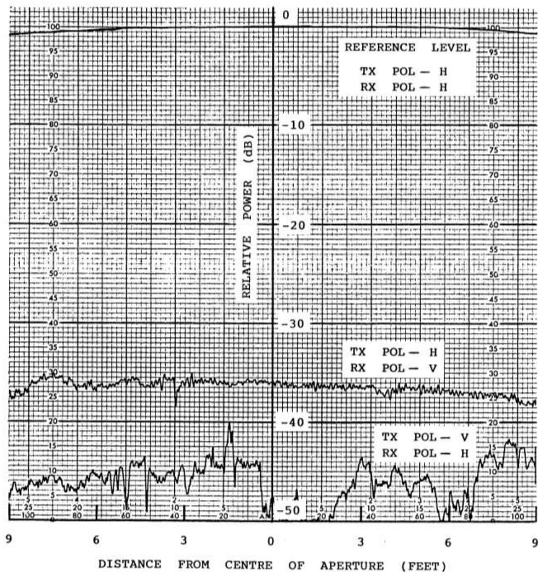
Figure 2.7 Family of polarization patterns as a function of source polarization angles at 22.5° angular spacing at 2.9 GHz for source height at 1.06 m
