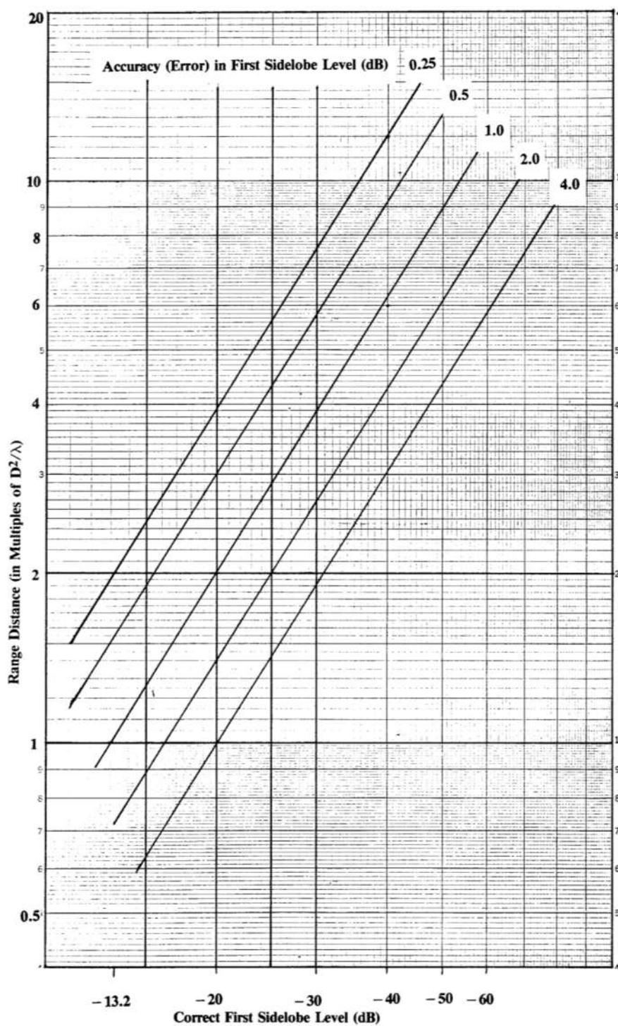
Figure 6.3 First sidelobe change versus normalised far-field distance for various first sidelobe design levels (note onset of shoulders)
