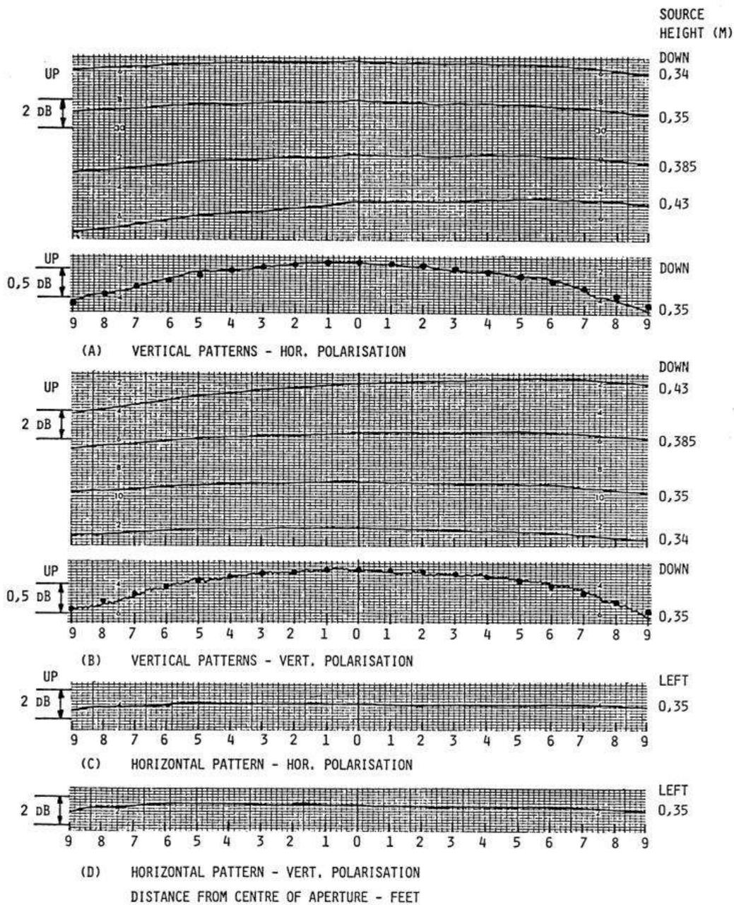
Figure 2.6 Measured cross polarization in the vertical plane over 5.5 m height at 9.6 GHz for source height of 0.35 m (1 foot = 305 mm)
