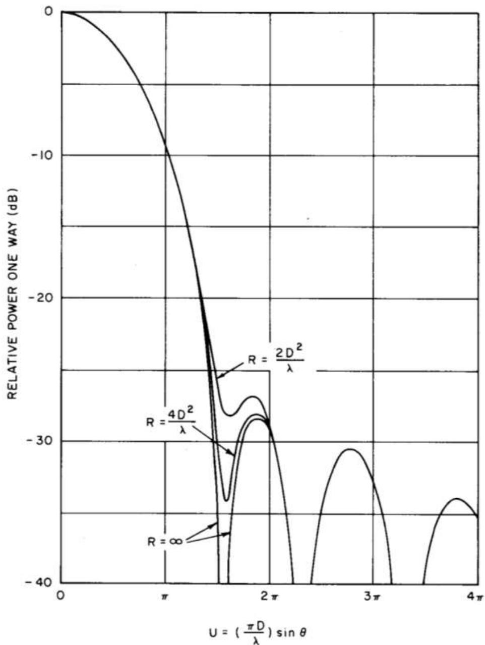
Figure 6.2 Range distance required for measuring the correct first sidelobe to the accuracy (error) stated on the straight lines
