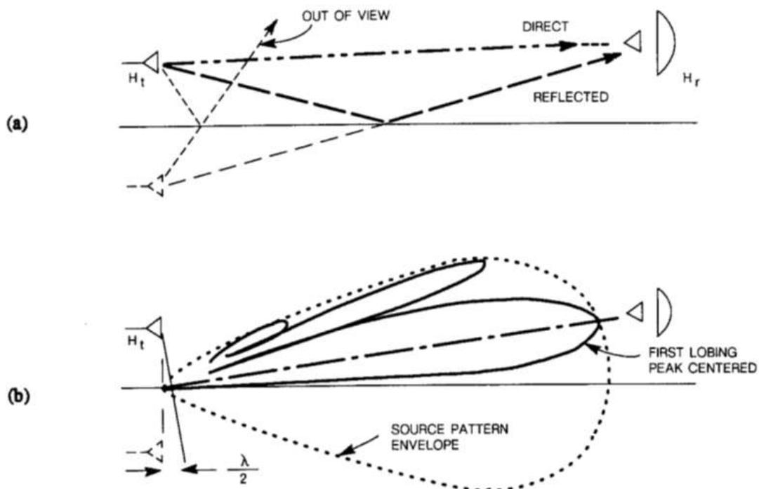
Figure 2.3 Taper in ground reflection range test zone (a) cosine variation, (b) edge taper as a function of the ratio of test antenna size size and height at centre of test zone
